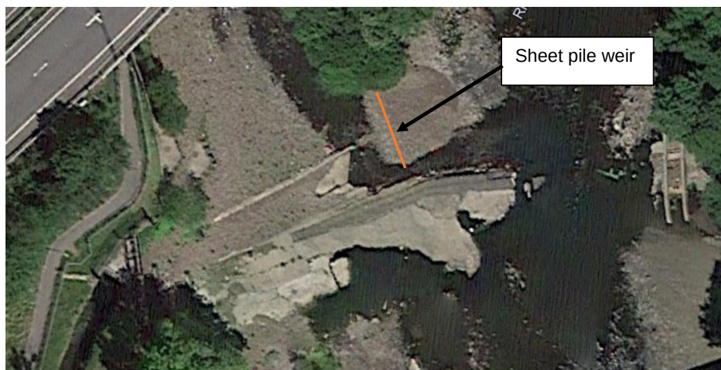
Figure 7 – Potential location of sheet pile weir
